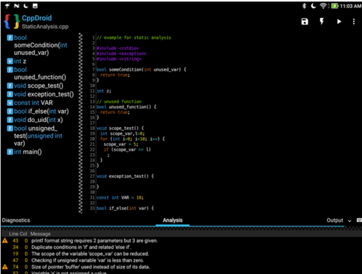
FIGURE 2-13: Use an example to see how the static analysis feature works.
